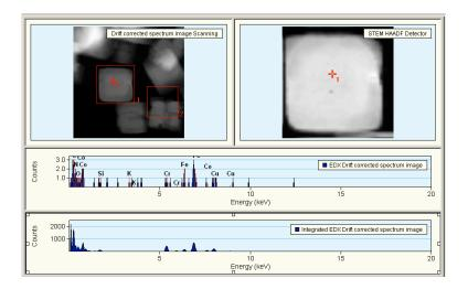
8.9. Select the sum spectrum and then select auto ID it to automatically identify the different peaks (this is usually sufficiently accurate) in the sum spectrum; you can also select KLM labels button to further characterize the peaks by transition.
