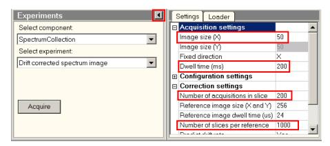
8.5. In the "Experiments" control panel, select "Acquire" to start collecting the spectrum image; after each spectrum at each point is collected, it will be displayed below the STEM image in TIA (the final spectrum shown will be the one collected from the last point in the defining region).
