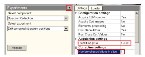
6.5. In the "Experiments" control panel, select "Acquire" to start collecting the spectra at the defined positions; after each spectrum is collected, it will be displayed below the STEM image in TIA (the final spectrum shown will be the one collected from the last point).
