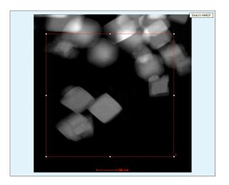
5.3. In Microscope Control, navigate to the panel, select "Acquire" to collect a survey spectrum from the defined area (outline will turn green); adjust the "Live time" (the time the detector is actively collecting X-rays) as needed (after starting the acquisition); the survey spectrum will appear below the STEM image in TIA and automatically update until complete.
