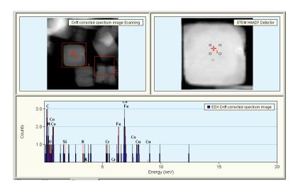
8.7. To generate the spectrum images for the elements of interest, the data must first be saved and TIA must then be expanded to analysis mode; select from the lower information panel; the button will change to and TIA will be in analysis mode.
