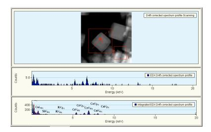
7.10. Select the periodic table button ; a periodic table dialogue box will pop up. Select the "ROI" tab to choose which elements will or will not be used to generate the profiles. Each time you select an element, you can select which X-ray peak(s) to use for mapping by selecting from the buttons
