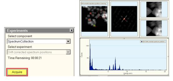
6.6. Once acquisition is complete and you want to view the individual spectra collected at the different points, you must first hide the beam position markers. To do this, simply right click on a beam position marker and select "Hide Object" and repeat for all remaining beam markers.
