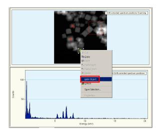
6.7. In TIA, select the image position marker tool and click anywhere on the image; then hold down the "Alt" key and click and drag it onto the spectrum below the image (the actual dark blue portion, not the background); the marker will now snap to a beam position marker and the spectrum for that point will appear. You can now simply click and drag the image position marker and it will snap to all the beam position markers and show the spectrum for each position.
