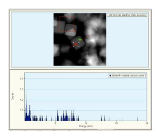
7.7. To generate the profiles for the elements of interest, the data must first be saved and TIA must then be expanded to analysis mode; select from the lower information panel; the button will change to and TIA will be in analysis mode.
