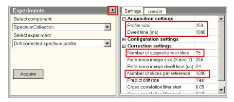
7.5. In the "Experiments" control panel, select "Acquire" to start collecting the spectrum profile; after each spectrum at each point is collected, it will be displayed below the STEM image in TIA (the final spectrum shown will be the one collected from the last point in the profile).
