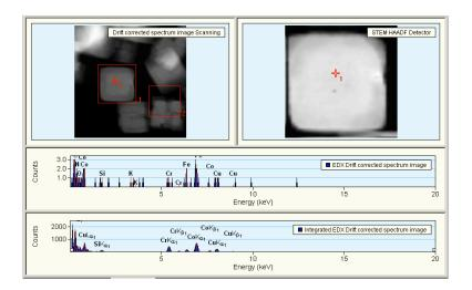
8.10. Select the periodic table button ; a periodic table dialogue box will pop up. Select the "ROI" tab to choose while elements will or will not be used to generate the spectrum images. Each time you select an element, you can select which X-ray peak(s) to use for mapping by selecting from the buttons.
