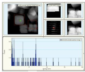
8.6. Once acquisition is complete you can view the spectrum collected at any point in the area used for spectrum imaging; simply click and drag on the image position marker tool in the area (you do not need to add a new marker) and the spectrum collected at that position will be shown below.
