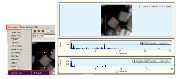
7.9. Select the sum spectrum and then select auto ID it to automatically identify the different peaks (this is usually sufficiently accurate) in the sum spectrum; you can also select KLM labels button to further characterize the peaks by transition.
