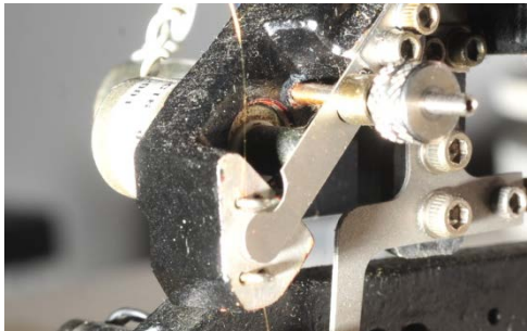
The EFO wand solenoid, which moves the wand under the wire during the ball making process; this solenoid can be actuated by hand
