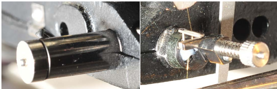
The wire tension clamp and solenoid, the clamp loosens to freely feed wire between bond phases with a set tension that straightens the wire as it is fed.
